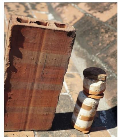
Fig. 5. Core drilling on the vault and stratigraphic composition.
