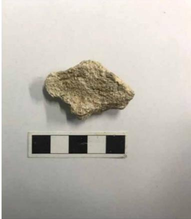
A photograph of a small, irregularly shaped, light-colored mortar sample. The sample has a rough, porous texture. Below the sample is a black and white scale bar for reference.                                                                                   |
