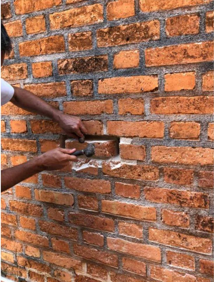
A photograph showing a person's hands using a hammer and chisel to carefully remove a sample from a brick wall. The bricks are reddish-brown and set in a grey mortar. The person is wearing a white shirt. The sample being removed is a small, irregular piece of material from the mortar joint. |
